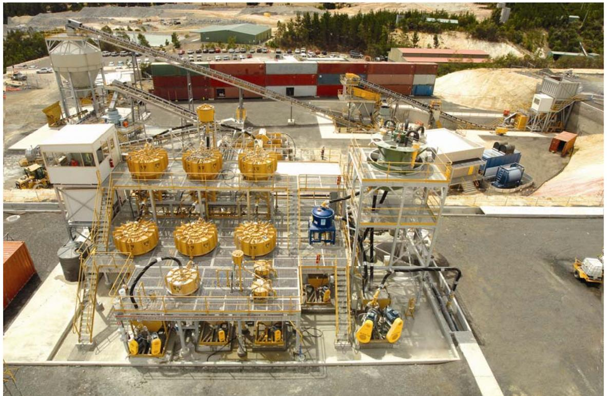
The complete Woolshed Gully gold processing plant - designed and installed by Gekko.
