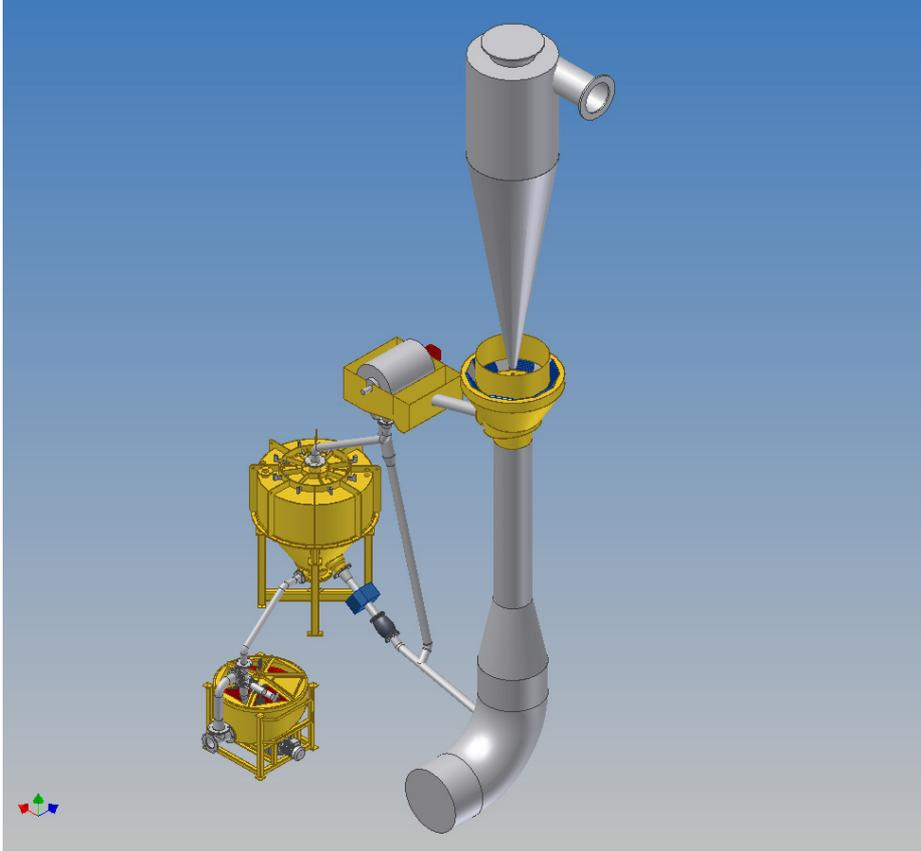
**Figure 4: General Arrangement of Gravity Circuit designed for South African Conditions**
