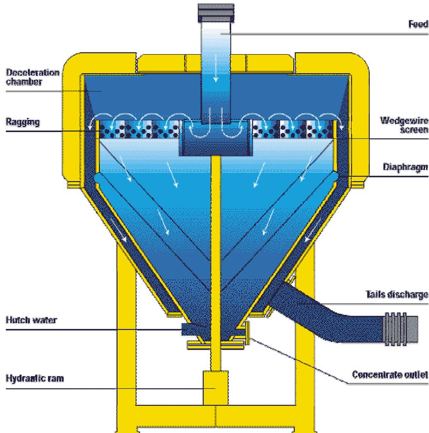
**Figure 1: Cross sectional view showing overview of an IPJ**
