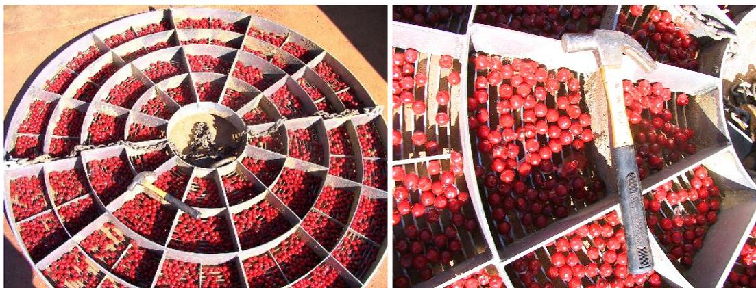
**Figure 7: IPJ diamond screen and synthetic ragging**
