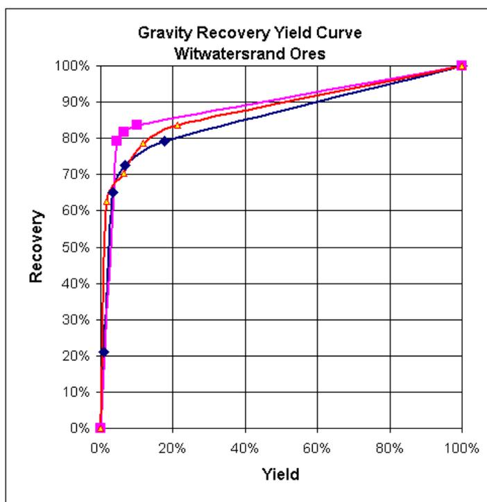
**Figure 3: Gravity Yield Curve on Various Witwatersrand Ores**
