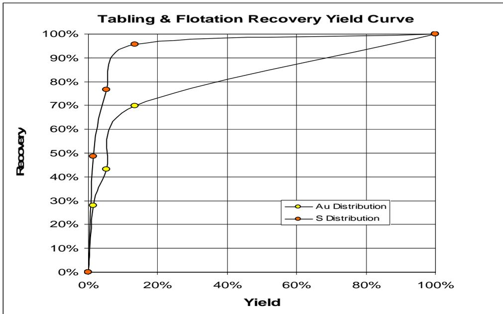
Figure 3: Tabling (gravity) and flotation results for Bong Mieu ore
