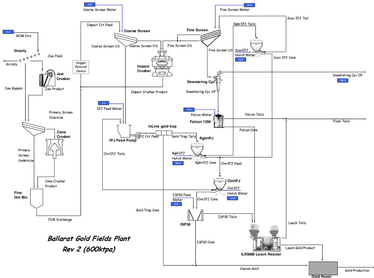
Figure 15: LIMN® model of the overall BGF Circuit (stages 1 and 2)
