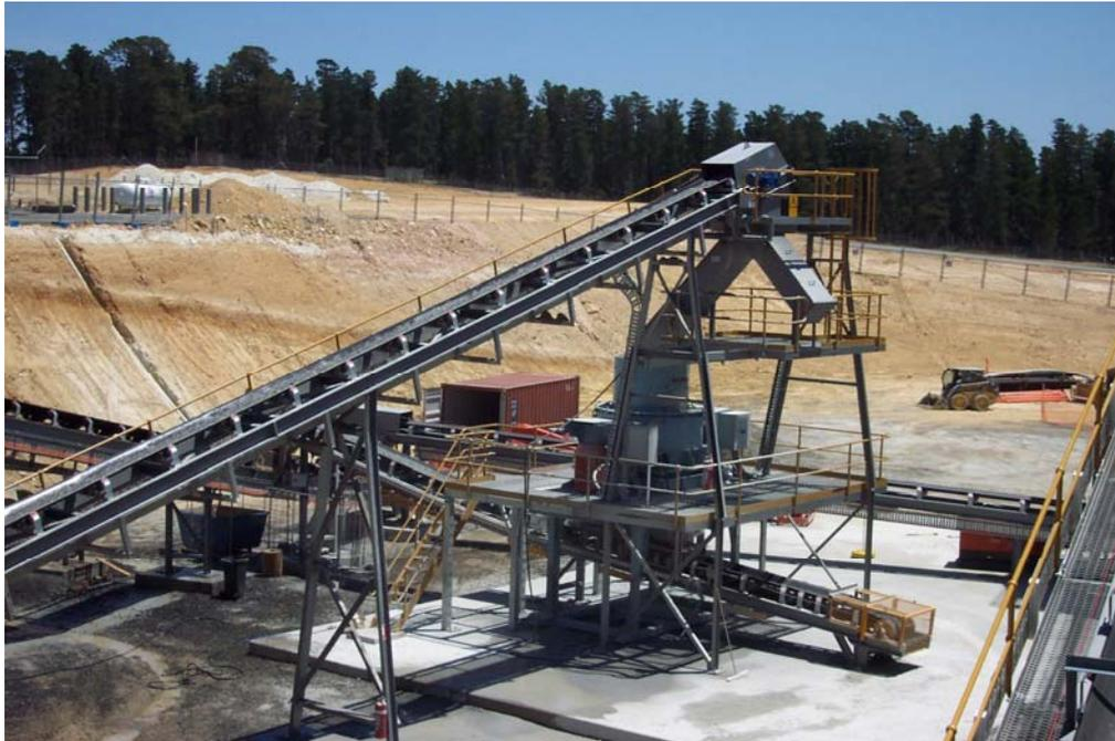
Figure 14: Vertical Shaft Impactor (VSI) and space for second VSI or HPGR
