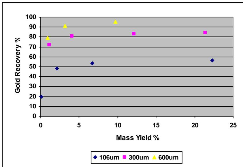
Figure 6: Affect of Grind Size (P100) on Gravity Recovery for BGF Ore Sample
