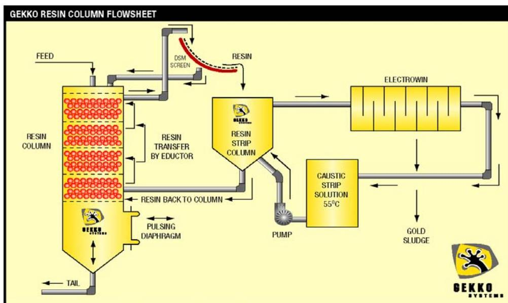
Figure 5: Gekko Resin Column and Strip circuit schematic as used at Bong Mieu
