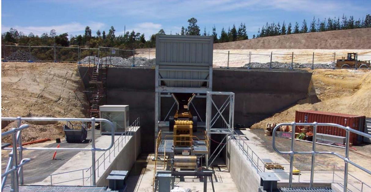
Figure 10: Jaw and cone crusher installed in a 3 metre recess to reduce noise emissions
