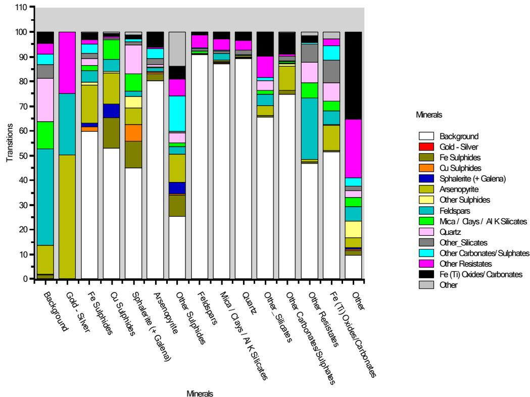
Figure7: QEMSCAN Bulk Mineral Associations of BGF ore after Impact Milling to a P80=1.2mm
