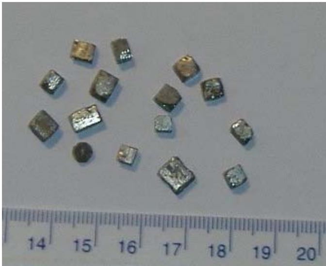
Figure 12: Arsenopyrite crystals recovered in the IPJ concentrate post VSI crushing.
