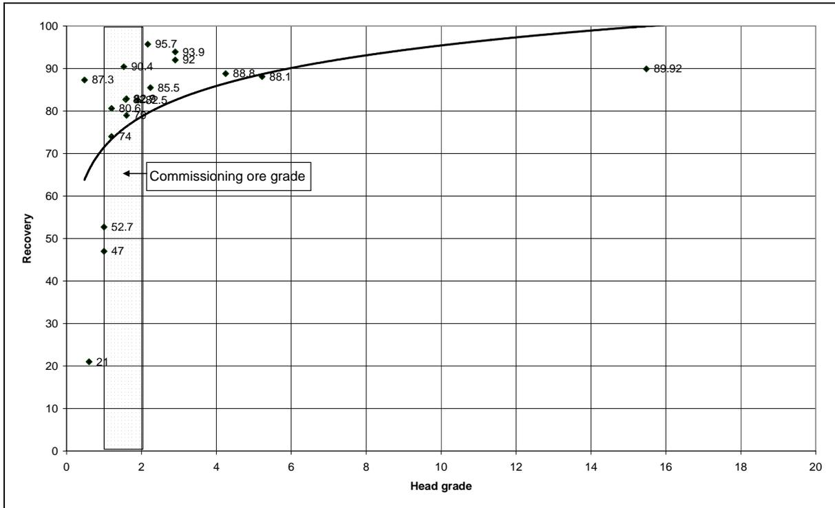
Figure 13: Gold Recovery to concentrate versus head grade for Ballarat East Ore
