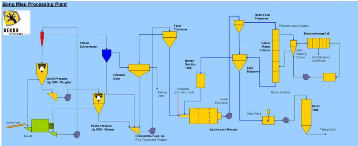
Figure 4: Bong Mieu Processing Plant Flowsheet (Post-Crushing)
