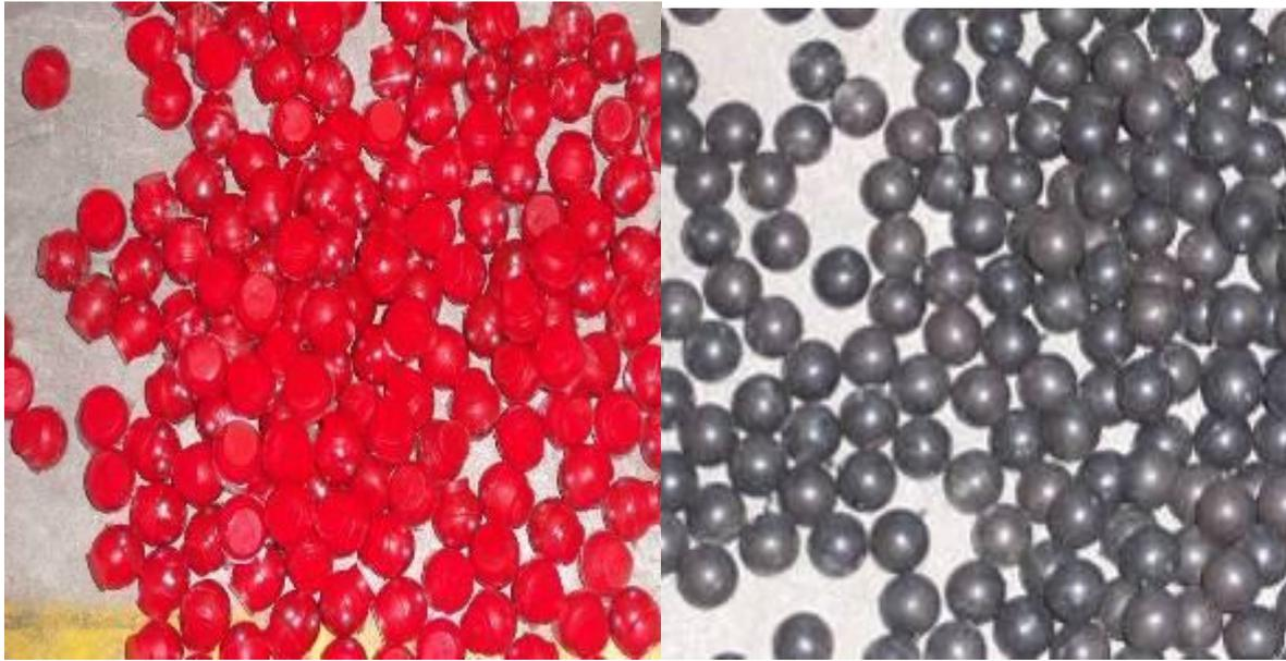
Figure 9: Gekko Polyurethane (Red) and Ceramic ragging
