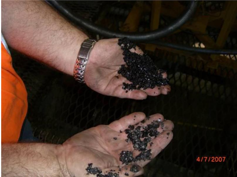
Figure 14: Floats (top) and Sinks (bottom) from an IPJ600 treating Australian -6mm coal
