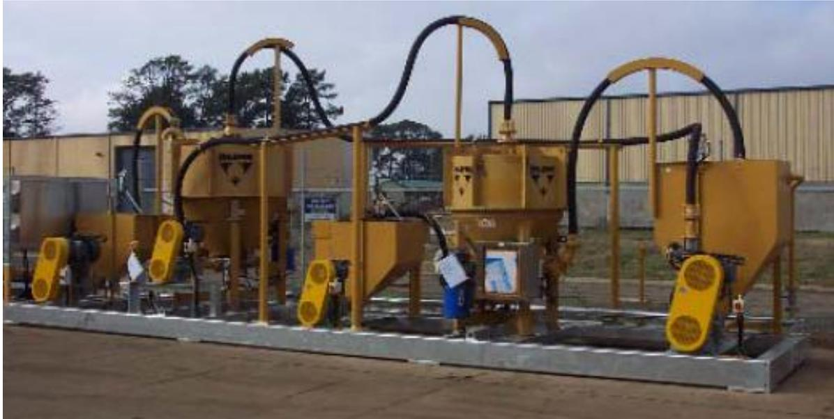
Figure 3: Two IPJ's installed in a gold and sulphide recovery application with products pumped.
