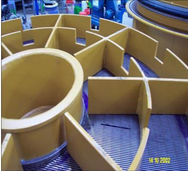
Figure 11: Bed drains to stop the build-up of heavies in IPJ beds.
