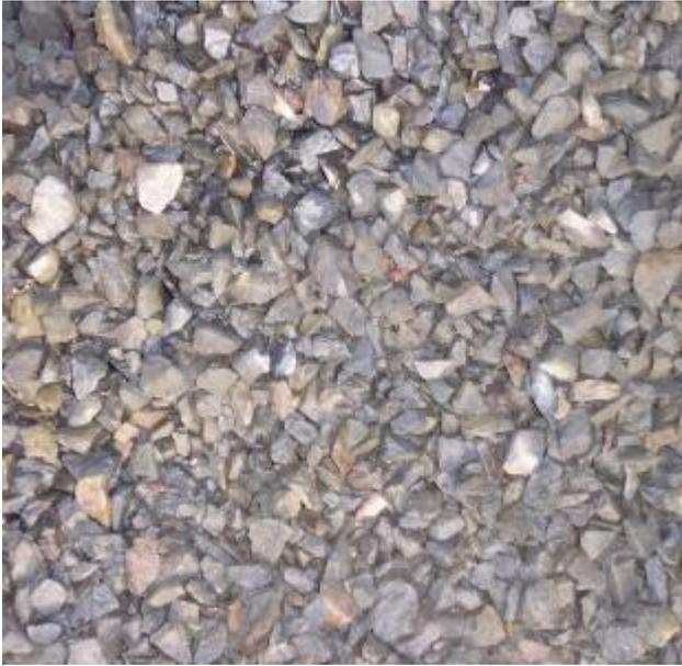
Figure 7: Naturally occurring Magnetite Ragging.
