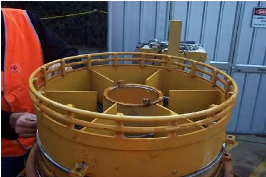
Figure 10: Ragging retaining screen
